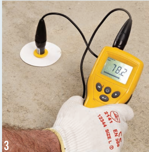
3 Insert the humidity probe. Readings above 75% RH require treatment.
