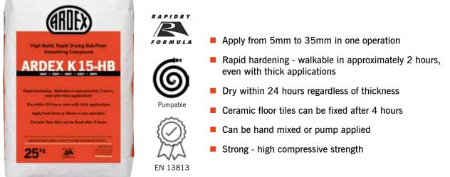
**ARDEX K 15 HB** is an advanced and versatile high build levelling compound designed for applications from 5mm up to a maximum of 35mm. It is virtually tension free and is designed to rapidly level uneven, hard subfloors.
