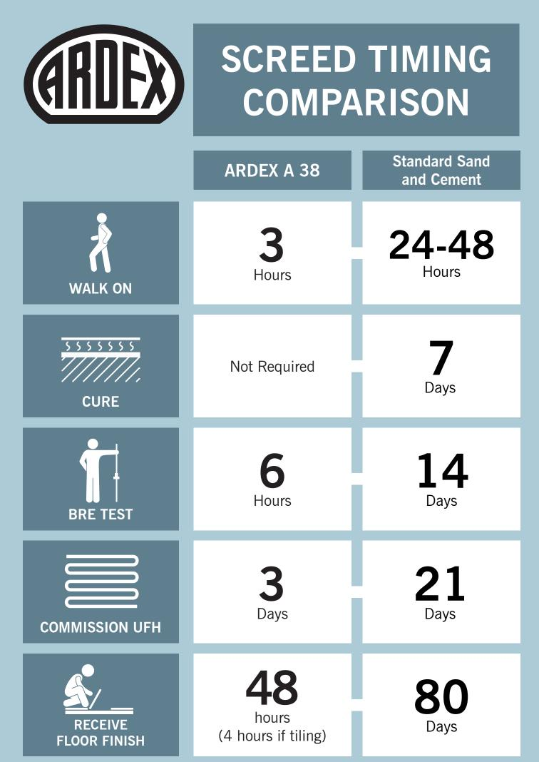
Note: Standard sand and cement timings in accordance to British Standards BS 8203 Installation of Resilient Floor Coverings
