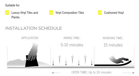
Times dependent on the absorbency of the subfloor and site conditions.
