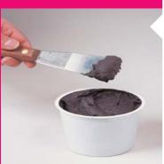
Mix a small amount of ARDEX WPC to a slump free consistency, as shown in picture 2, for filling holes, gaps and joints. The working time is approximately 45 minutes at 20°C.
